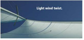
when the boat luffs up. If it backs in the top first the lead position is to far aft and vice versa. Halyard tension should be lightly applied. In really light winds small wrinkles should be seen running away from the forestay.
